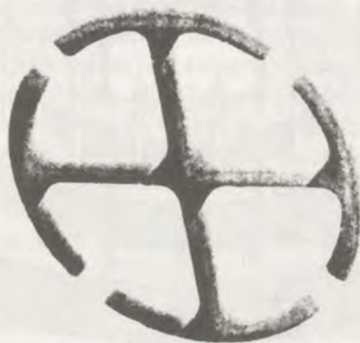
Figure 4.8 Spinneret plate for the production of hollow fibres. LIGA technique, Ni, diameter of 20\ \mu\text{m}
