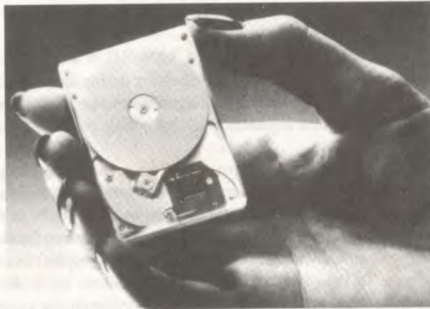
Figure 5.7 The HP Kittyhawk PSM 1.3 inch disk drive module has 21.4 Mbytes of storage space Source: Hewlett Packard
