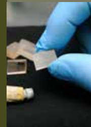
Crosssamples from art masterpieces moulded in high glass plates ready for investigation with electron X-ray. The historic paint tube at the bottom is from the personal collection of M. Cotte, artist I. Montero/CAIF.
