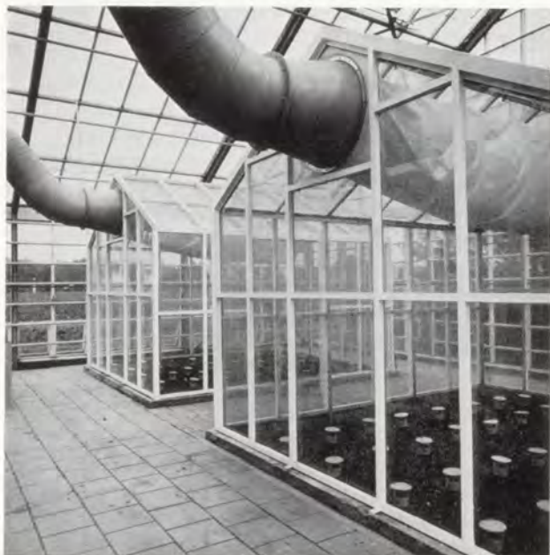
Figure 1 - Chambers for short term experiments with plants exposed to relatively high concentrations of test gases.
