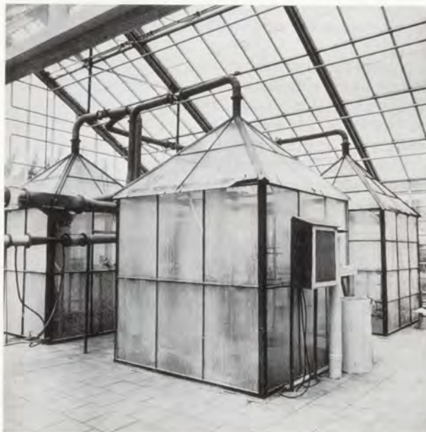
Figure 2 - Exposure chambers for the administration of very small gas concentrations to plants during a whole growing season.
