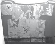
*Picture of an unpackaged RF-MEMS switch.*
