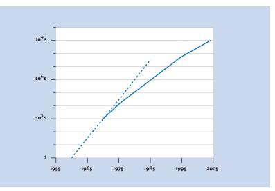
Two technological developments have paved the way for Moore's Law: minimum pattern dimension (decreasing) and wafer size (increasing). In 1965, manufacturing relied on 25-mm substrate wafers; now it is 300 mm. At the same time, the smallest patterns on these wafers have been reduced from several times the size of a red blood cell (6-8 micrometre) to that of the common cold virus (20 nanometre).
