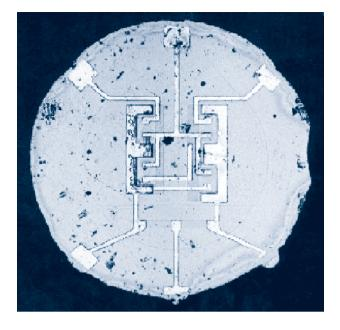
In that same year 1959, Texas Instruments' engineer Jack Kilby submitted a patent request called 'Miniaturised Electronic Circuits', on making resistors and capacitors in semiconductor technology together with transistors on one and the same silicon substrate. A concept which at that time existed only on the drawing table — Figure 1 shows the demonstrator realised one year later — but what became quickly known as the integrated circuit (IC).
