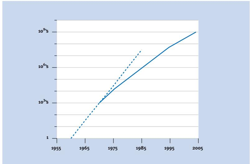
Two technological developments have paved the way for Moore's Law: minimum pattern dimension (decreasing) and wafer size (increasing). In 1965, manufacturing relied on 25-mm substrate wafers; now it is 300 mm. At the same time, the smallest patterns on these wafers have been reduced from several times the size of a red blood cell (6-8 micrometre) to that of the common cold virus (20 nanometre).
