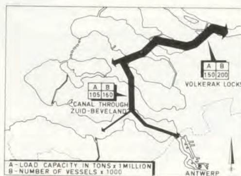
Figure 42 - Shipping flows between the West Scheldt basin and the Hollandsch Diep (in 1975, before the opening of the Scheldt-Rhine link).
